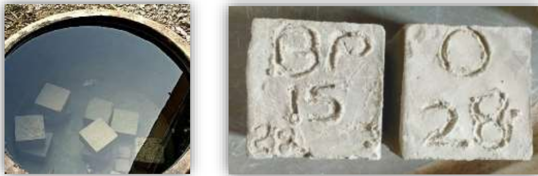
Fig 6. Curing of cubes
