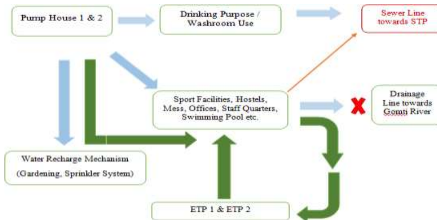
Fig. 3.3 Flow Chart of Water Supply System
