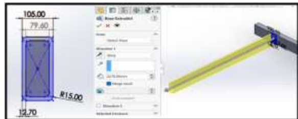
Figure 12 dimensions of hallow section cross member
