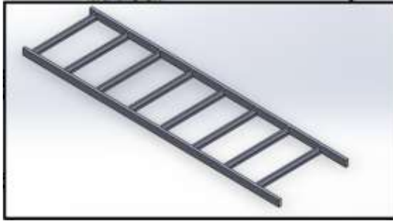
Figure 13 isometric view of hallow-section cross member
