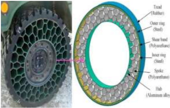
Figure 2 honeycomb structure nomenclature
