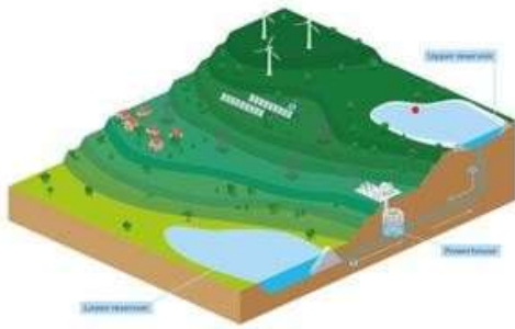
Fig.2.2 Pumped Storage Hydropower
