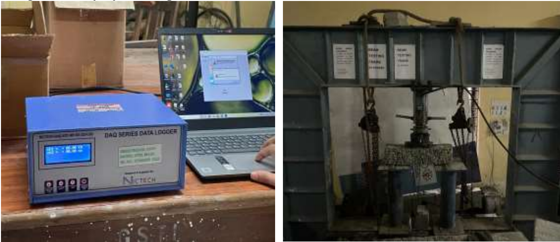
Fig 13: Images show Data logger, Laptop and the Set-up used for testing of specimens. Stress-Strain Curve for M40 and M65 grade Cylinders:
