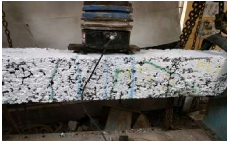
Figure 25 Failure Pattern of Beam under Cyclic Loading test
