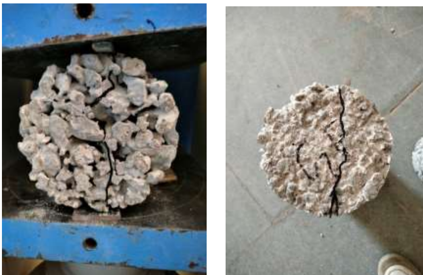
Figure 24 Failure Pattern under Split Tensile Strength test
