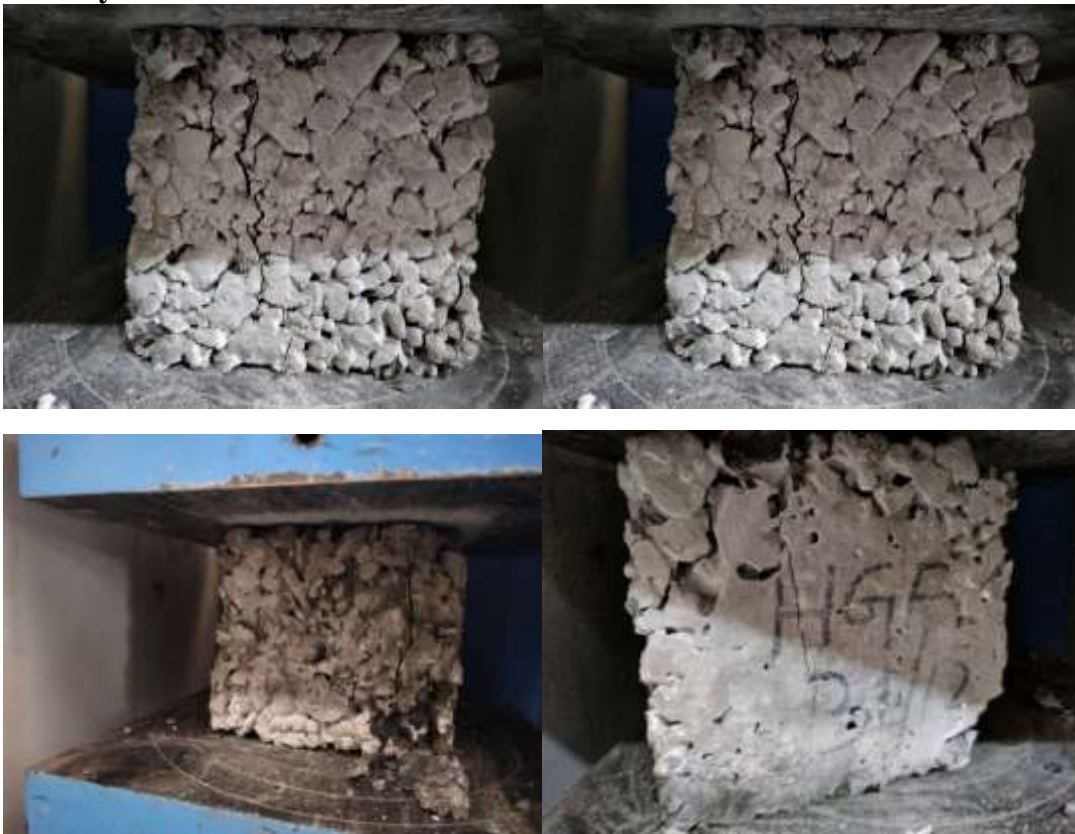
Figure 22 Failure pattern of pervious concrete cube under CTM
