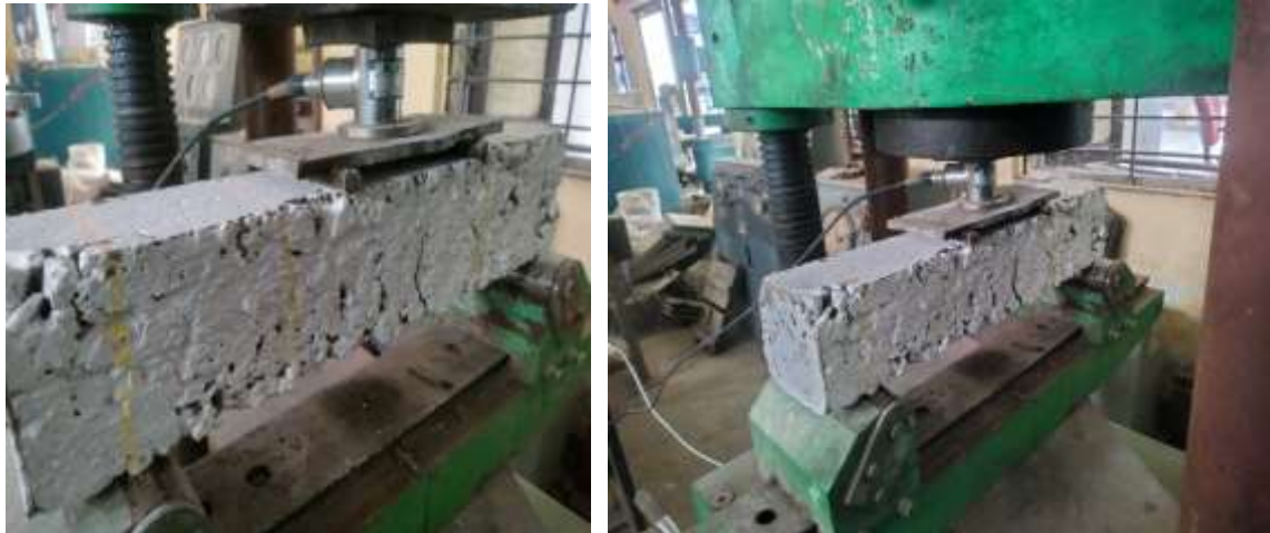
Figure 25 Failure Pattern of Beam under Flexural Strength test
