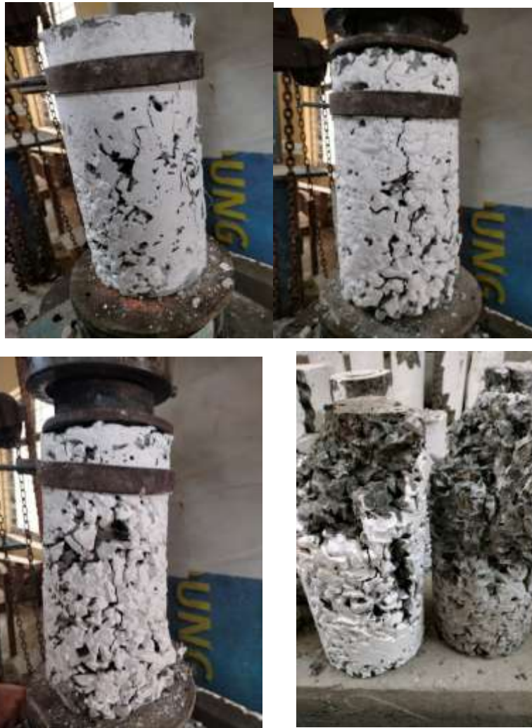
Figure 23 Failure pattern of pervious concrete Cylinder under cyclic loading
