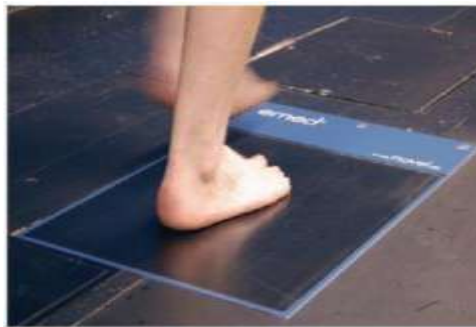
Figure 1.1: Plantar pressure measuring device
