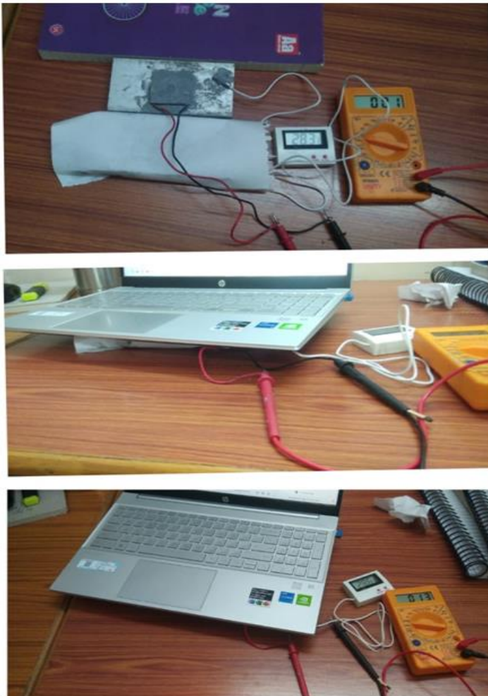
FIGURE 10:Working Process in Flexible thermometric device to harvest waste heat from the laptop
