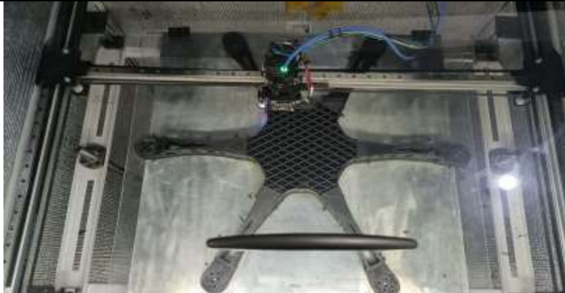
Figure.4. Manufacturing of Hexa-Copter Sliced using 3D printing
