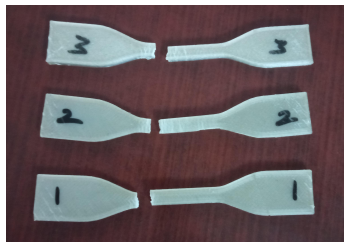
Figure 14 Tensile Test Samples
