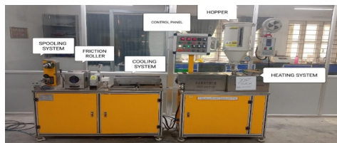
Figure 10 Single screw filament extrusion
