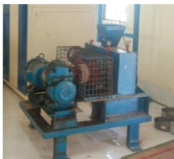
Figure 4 Roll Crusher Figure 5 Ball Milling Figure 6 Powdered capra hircus bone
