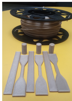
Figure 13 Printed Test Samples
