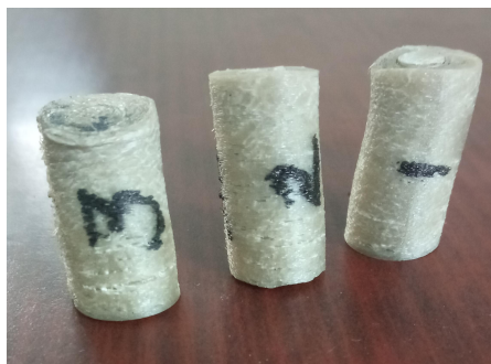
Figure 15 Compression Test Samples
