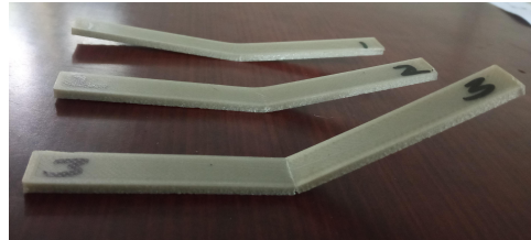
Figure 16 Flexural Test Samples
