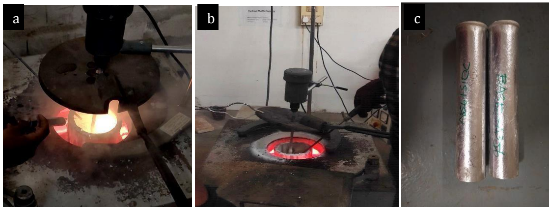
Fig 5.2 (a) and (b) stir casting of A356 + 2.5% SiOC Fig 5.3 Test specimens
