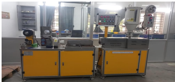
Figure.4: Single Screw Filament Extruder machine setup
