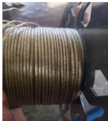
Figure 5: PLA – Blepharis maderaspatensis powder obtained as filament
