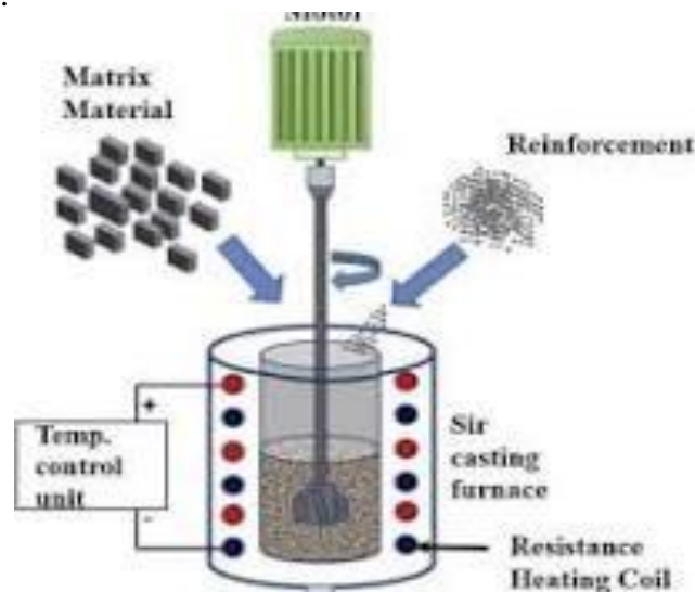
Figure 1: Stir Casting Setup [19]
