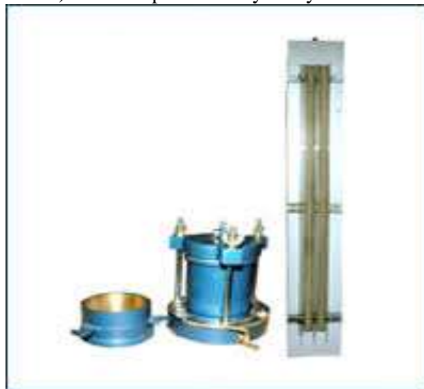
Fig 5: showing permeability test apparatus
