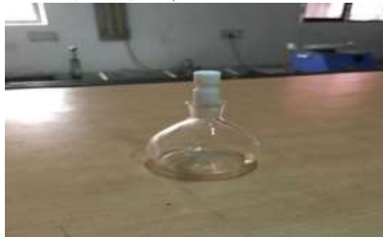
Fig 3: showing density bottle method apparatus used for determining Specific gravity
