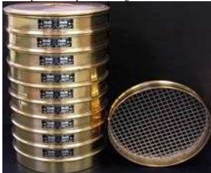
Fig 4: showing sieves used for sieve analysis test
