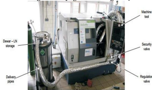
Figure 2. Cryogenic Machining Setup [20]
