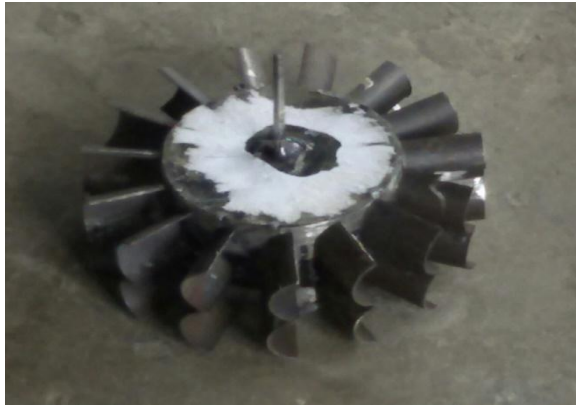
Fig-7 Pelton Wheel Turbine
