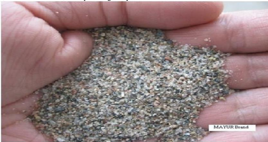
Figure 3 Coarse sand of Zone II
