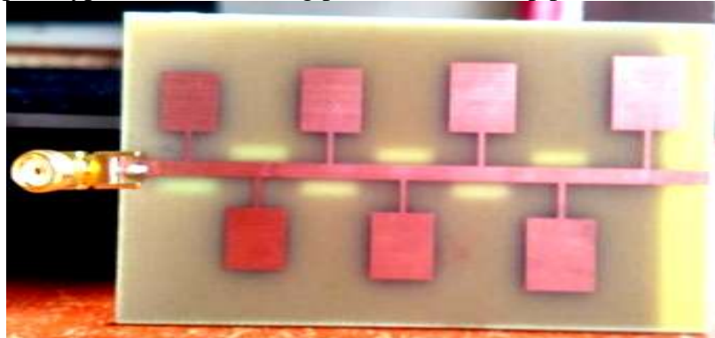
Fig 4. Fabricated design of 7-element Log periodic Microstrip Patch Antenna array with DGS
