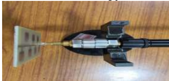
Fig .17. Measurement set up of 7-element Log periodic microstrip Patch antenna array without DGS
