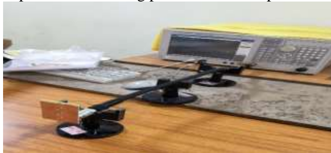
Fig 18. Measurement set up of Log periodic microstrip Patch antenna array with DGS
