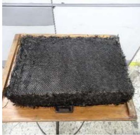
Fig. 3: 3D Pierced Fabric (8H Satin Weave) Preform
