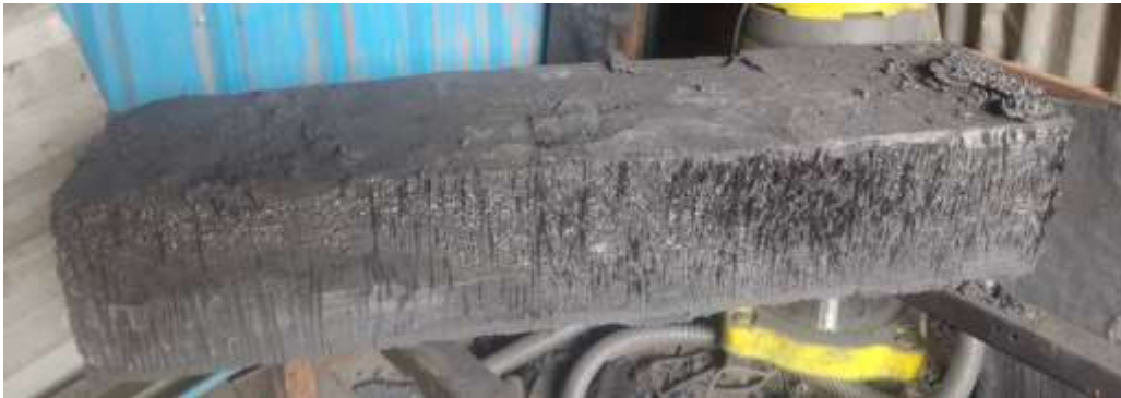
Fig.3: Fabricated 3D PF C/C composite billet
