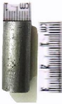
L=30mm, D=10mm Figure 3:Sample specimen
