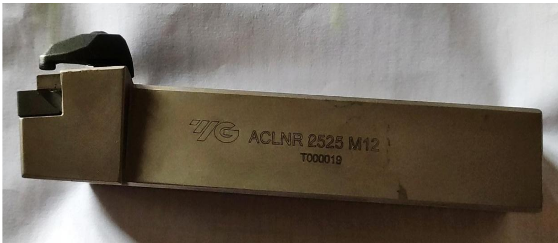
Figure 2.2: Tool holder (YG make)
