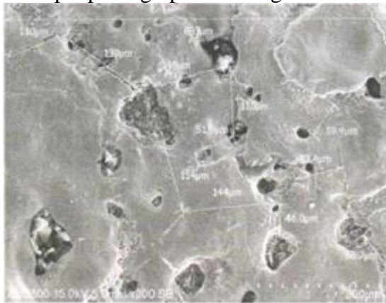
Figure 6: SEM photo of machined workpiece at current 10A; pulse on time 800 \mu\text{s} ; duty factor 2, gap voltage, 20 V (without powder). Total Average crack length=1126.5 \mu\text{m} Area = 633 \times 633 = 400689 \mu\text{m}^2 Crack density = 1126.5/ 400689 =0.0028 \mu\text{m}/\mu\text{m}^2
