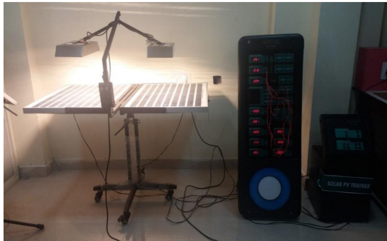
Figure 2.1 System setup to determine I-V characteristic at different irradiation level
