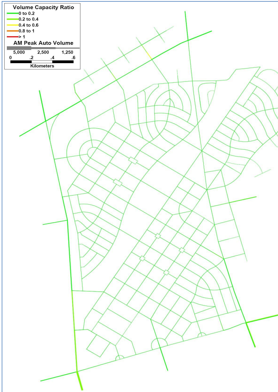
Figure 1: Morning peak auto volume colored by volume capacity ratio. All links have v/c ratios of less than 0.8, indicating the roads are significantly under-utilized.
