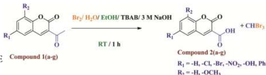
Scheme 3 — Haloform reaction of compound (1) to yield corresponding carboxylic acid
