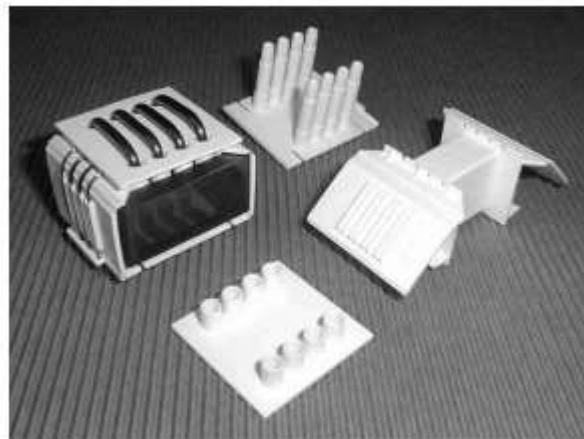
Fig.7: Transformer of the resonant 500W DC-DC converter using "bow winding" technique (shown here for N1=4) for direct PCB mounting and components of the coil former.
