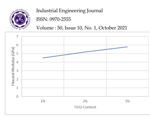
The observed improvements in tensile and flexural properties with increasing TiO2 content align with findings from previous studies, showcasing the reinforcing effects of TiO2 in epoxy composites (Smith et al., 2018; Wang and Zhang, 2019). The increased strength and stiffness are attributed to the efficient load transfer and improved interfacial adhesion between the TiO2 nano-fillers and the epoxy matrix.
