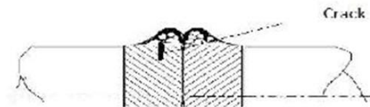
Figure 6: Crack at the sharp edge transitional area to weld flash
