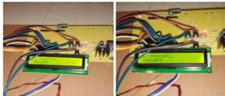
Fig.2 Experimental setup Ultrasonic sensor placed inside the dustbin is responsible for monitoring the level of garbage. The level detected by the ultrasonic sensor is shown on the LCD screen.
