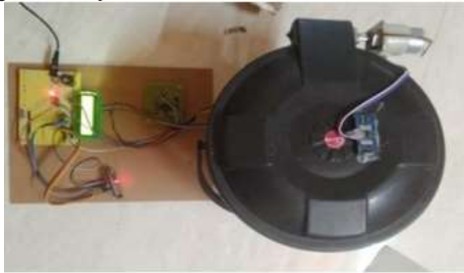
Fig.2 Experimental setup Ultrasonic sensor placed inside the dustbin is responsible for monitoring the level of garbage. The level detected by the ultrasonic sensor is shown on the LCD screen.
