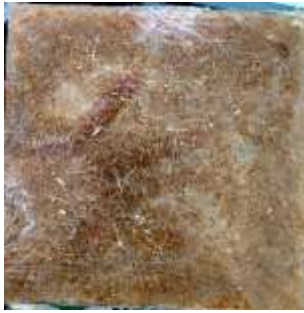
Fig: 184gms Epoxy + 116gm Hardener + 10gm coconut fiber Pictures representing the formation of the composite
