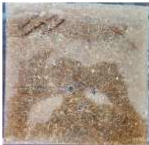
Fig: 184gms Epoxy + 116gm Hardener + 5gm coconut fiber Pictures representing the formation of the composite
