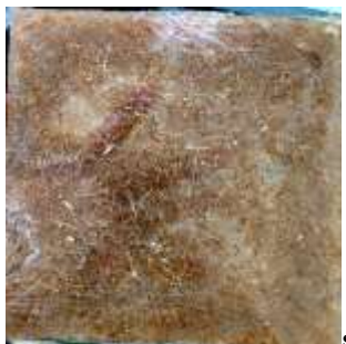
Fig: 184gms Epoxy + 116gm Hardener + 5gm coconut fiber Pictures representing the formation of the composite
