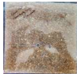
Fig: 184gms Epoxy + 116gm Hardener + 5gm coconut fiber Pictures representing the formation of the composite
