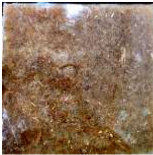
Fig: 184gms Epoxy + 116gm Hardener + 15gm coconut fiber Pictures representing the formation of the composite
