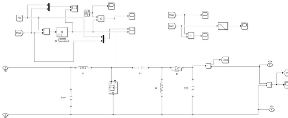
Figure 3: Subsystem of the SEPIC converter block
