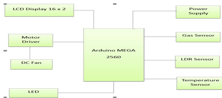
Figure 2: Block diagram to maintain warehouse condition
