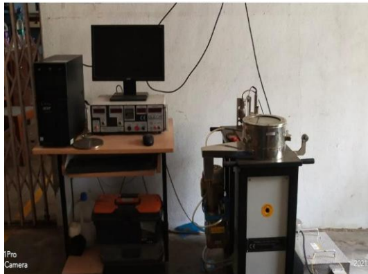
Figure 3: Setup of dry sliding wear test
