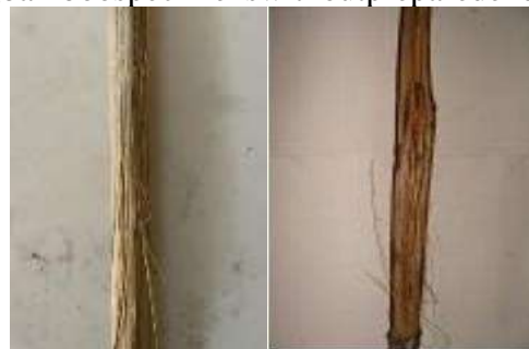
Fig. 3. Splitting failure of the bamboo specimen
