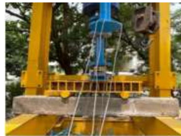
(b) Load the Specimen by Giving Axial Load
