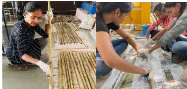
(a) Coating of epoxy resin (b) Glass fiber coating on the bamboo
