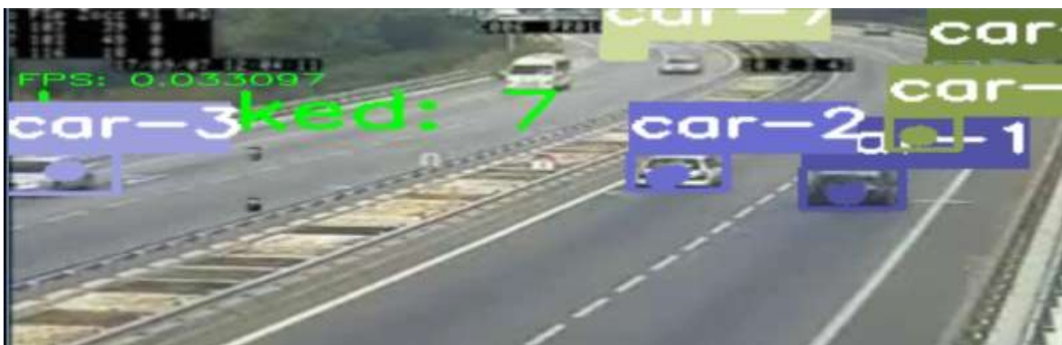
Fig 5. Detection and tracking of cars and trucks using YOLOV4 with DeepSORT algorithms.
