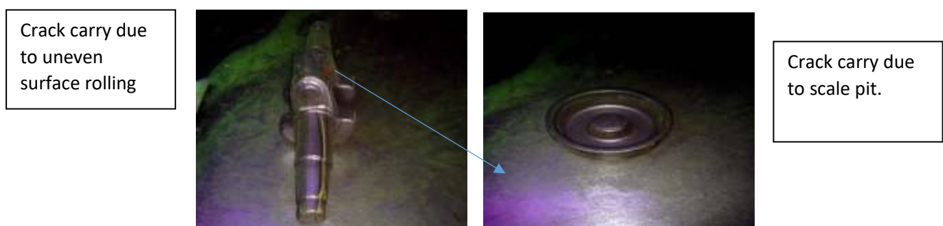
Fig 12 Crack Formation Job for Overheating and Rolling Operation.
