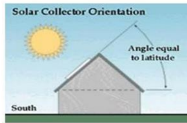
Figure 6: Stationary PV panel orientation[24]
