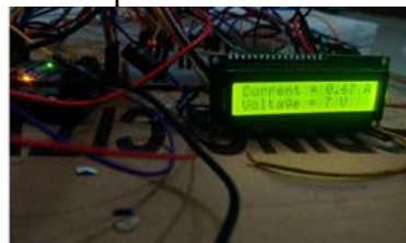
Figure 46: Output Voltage and Current under Low Light Condition
