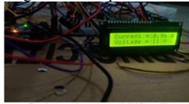
Figure 42: Voltage and Current Output of from the Solar Panel under High Illumination of Sunlight.
