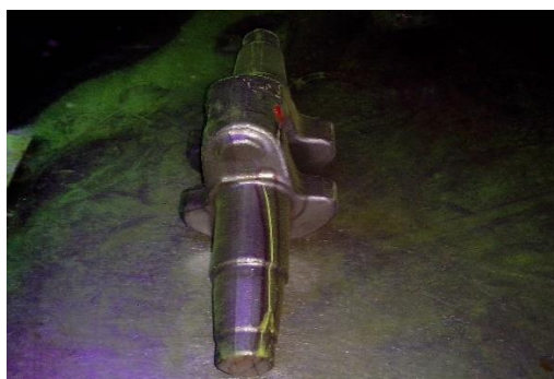
Fig 05 Non-Uniform Deformation Crack
