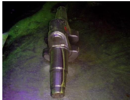
Fig 05 Non-Uniform Deformation Crack
