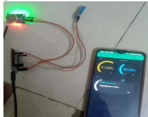
Fig.15: If Flammable Gas is there the Notification Send
