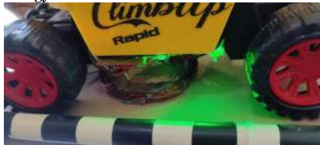
Fig 7: The power is transfer through the windings
