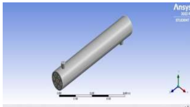
Fig 3.1. 3D Modeling of shell and Tube heat Exchanger (Fusion 360)
