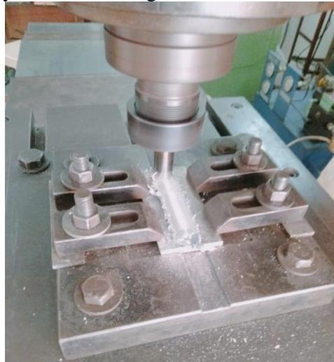
Figure 2: FSP Experimental Setup
