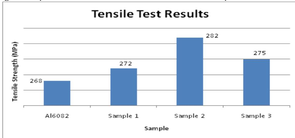
Figure 5: Tensile test results
