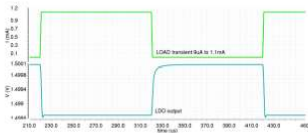
fig 10: load transient 9uA to 1mA in 5kHz
