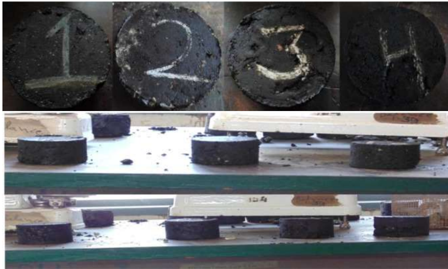
Figure 1 CRMB-60 mix pavement specimen with various height
