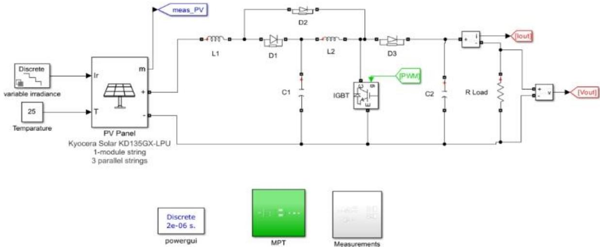
**Figure 6.** Proposed Design and simulation of PV connected Quadratic boost converter
