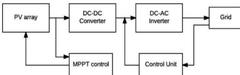
**Figure. 10.** Block diagram of a basic grid-connected PV system
