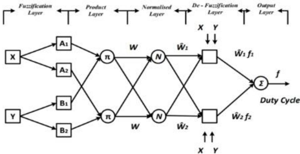
**Figure. 5.** Structure of ANFIS controller
