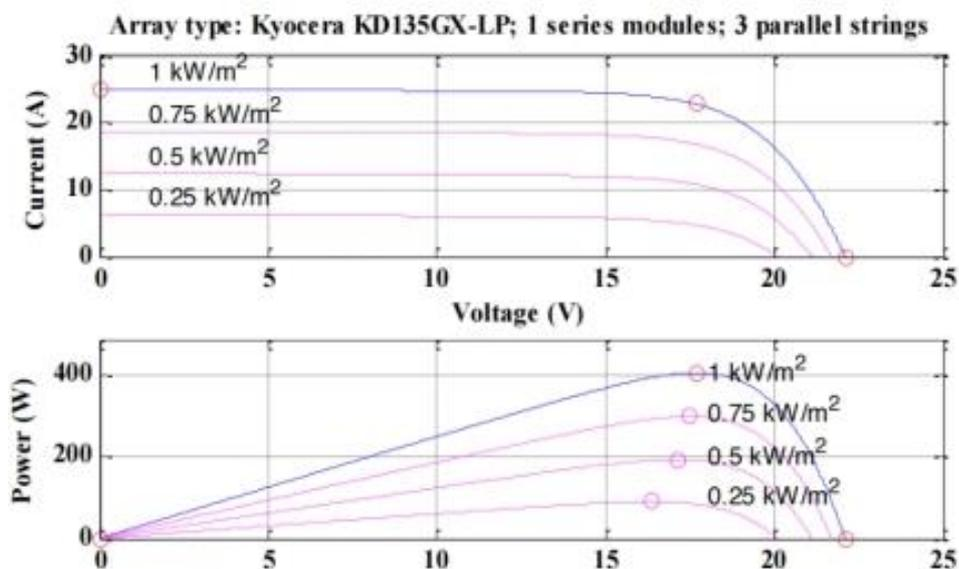
**Figure.7.** 400 W PV system P-V & I-V characteristics of Kyocera KD135GX-LP.
