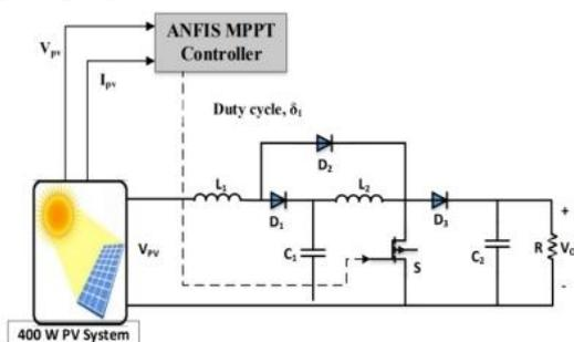
**Figure. 1.** Block diagram of the proposed system.
