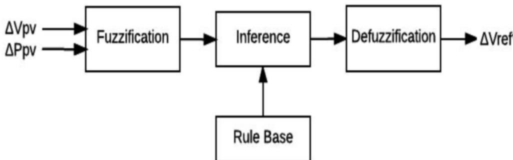
**Figure-4** Architecture fuzzy logic Controller
