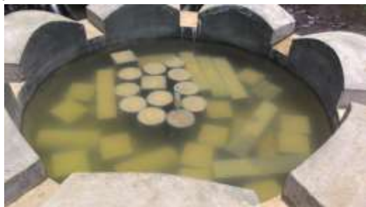
Figure-5.1.5: Shows Curing Tank TESTS ON HARDENED CONCRETE:
