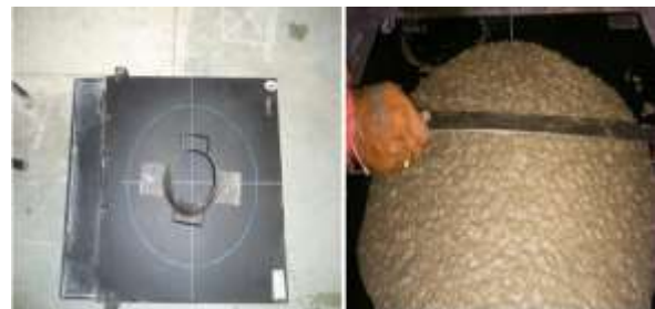
Fig. 3.2.3.1 Slum Flow Apparatus & Testing
