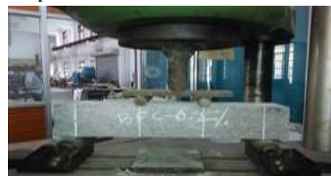
Fig. 3.5 Loading Arrangement for Load-Displacement Test
