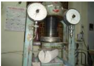
Fig: 3.2.6.2 Split tensile Test Set-Up
