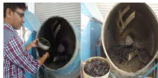
Fig. 3.3.1 Addition of Fiber to the SCC Mix Ultrasonic Pulse Velocity Test
