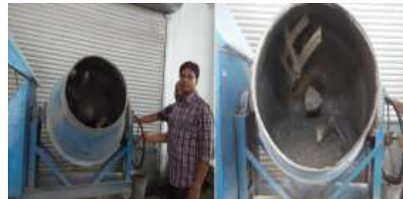
Fig.3.2.1 Concrete Mixture Machine & Preparation of SCC Mix
