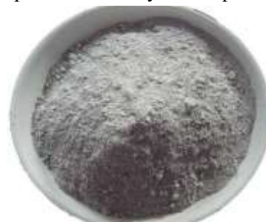
Fig2.2: Sample of silica fume used in concrete
