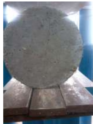
Fig 5.4: Split tensile test on cylinder
