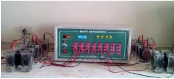
Fig. 5.7 (b) RCPT TEST
