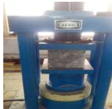
Fig 5.3: Cube compressive strength testing machine.
