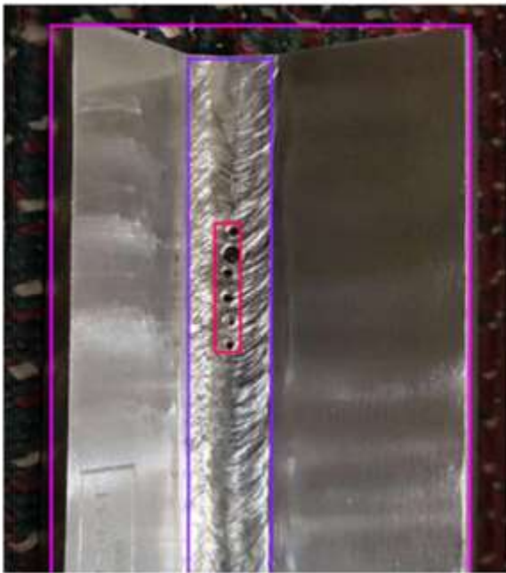
Fig 4(A): Image showing the porosity in corner joint Fig 4(B): Image showing spatter in butt joint
